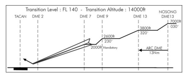
This view is the same as the plan view but viewed from the side which give the pilot the required altitude at specific points of the approach. Let's get back to the Chongju approach we used as an example for the DME ARC transition to the ILS.
