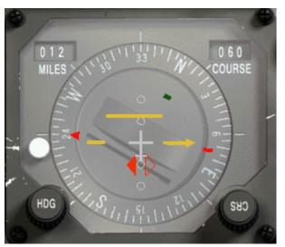
At point 1, the CDI started to centre. The station bearing pointer is still maintained on the nine o'clock position but I drifted a little toward the station since the DME is now reading 12 Nautical miles. The heading is now 330°. It's important to check the heading leaving the IAF, during the DME arc and certainly the exit DME ARC heading which here would be 230°+90°=320° if we were to continue the DME ARC to the ILS localizer. It's good practice to commit these reference headings to memory.
