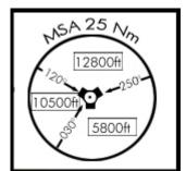
arrival headings. On this example, pilots should notice that the minimal safe altitude between arrival headings of 250° and 030° is 5800 feet MSL. The minimum safe altitude between arrival heading of 030° and 120° is 10500ft MSL and the last sector between arrival heading of 120° and 250° is 12800ft MSL. Basically, it means that we have high terrain at least 11000 ft on the northern sector and high terrain at least 9000ft high on the western sector.
