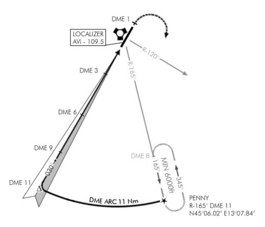
The approach track always starts at the IAF which stands for Initial Approach Fix and marked with a star on the chart. It is named as a fix, usually with a 5 letters name (here PENNY). Its position is given both in GPS coordinates and with a radial from a known tacan and the distance from the station (DME).
