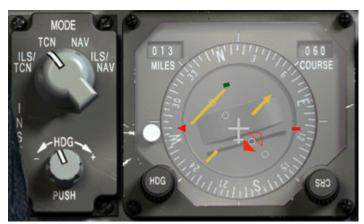
A short while after leaving NOSONG, the aircraft is slightly banking left so the red station bearing pointer remains on the 9 o'clock position – to remain at DME 13 from the station. The mode is set to Tacan and radial 060° is set in the course arrow. Note the heading which is 015° - the departure heading from Nosong was 030° (300°+90°=030°) so we already turned 15°
