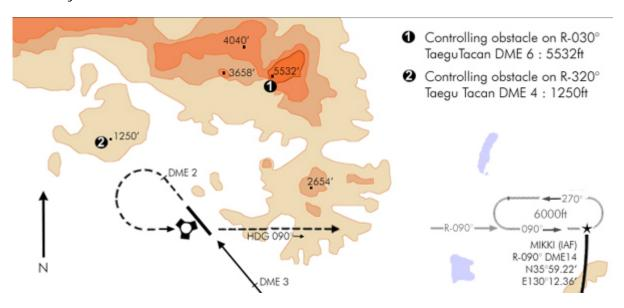
White area pictures terrain up to 999 feet. The lighter brown pictures elevations between 1000 and 1999 feet. The next shade between 2000 and 2999, and so on. The darker the shade, the higher the terrain.
