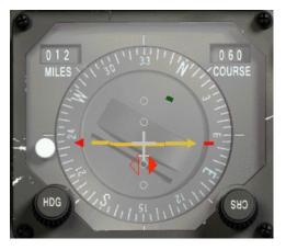
At point 2, the CDI is centred, it is now time to turn left to a 270° heading and switch the mode selector to TCN/ILS so the CDI displays the localizer instead of the tacan radial. This is really a step not to be missed because it induces some confusion as you will see on the next picture.
