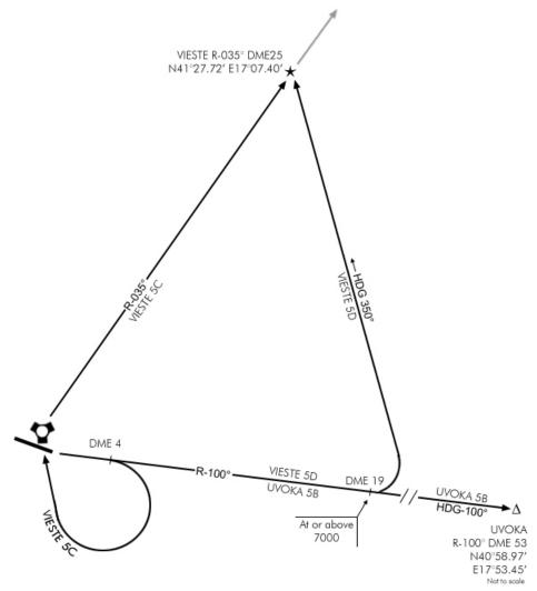
Let's consider Amendola departure. Amendola is an 11/29 runway and there are three different routes for each runway. Two different exit points in total. One in the North, on a
