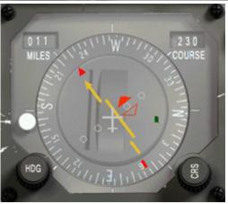
HSI with the course arrow set correctly on the 230° radial and with the CDI a notch to the right. Indeed, while setting it up, the aircraft got closer to the ILS (we are now at DME11) It's high time we make our final left line-up turn to get properly on the localizer. Luckily, we don't have any passenger on this flight.
