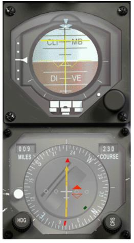
We are now at position 4, lined up properly with the localizer and waiting for the glidepath to come down on us. We are at DME 9 and should then be at 2800 ft as the side view of the chart instructs us. We should now start a descent of 800ft to pass DME 7 at 2000ft until glide interception.
