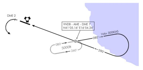
The VNDB point is placed along the runway centreline at a distance of 7 Nm from the airbase. As you noticed, the GPS coordinates of this specific point are given. This is good because with that information, we can set the VNDB as the last waypoint of the flightplan for instance. Through the UFC, select the last waypoint before landing and enter its new coordinates. Having done that, the waypoint can now be used as a virtual tacan if two conditions are met:
