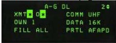
The Data Link pages are used to set your in-flight data-link settings. There are only two selectable options in the Air to Ground page: the transmit address and the FILL option.
