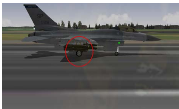
Figure 4 – The Element Line Up Position: View of aircraft in front (Note the Main Gear is in line so you can only see the one main wheel)
