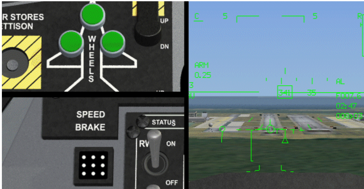
INTERCEPTING THE GLIDESLOPE - BRAKE OPEN AND GEAR DOWN
