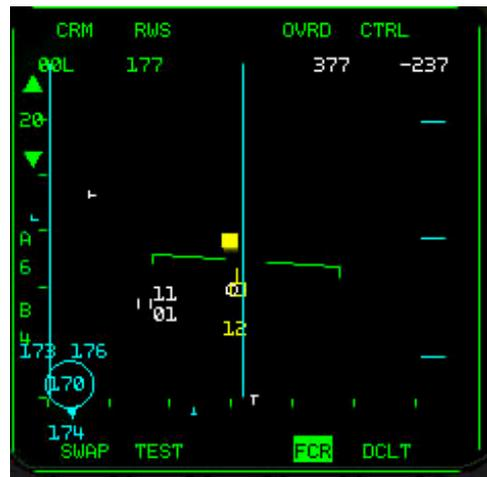
The final difference between this and the standard mode is the Dynamic Launch Zone (DLZ) scale will appear on the right of the radar screen when you have air-to-air missiles selected. This DLZ is sized to correspond to the range display in the radar screen, and you can use the range ticks to gauge
