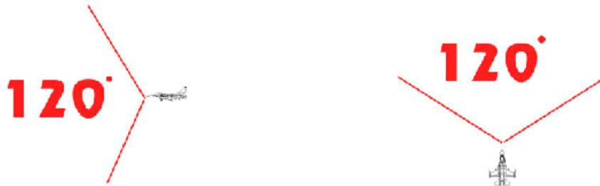
The AN/APG-68(V5) can look 120° by 120° in front of the aircraft, it cannot however cover all of this area at once, even if it could, it would not be very useful because of the time that it would take to accomplish a full scan. To get around this problem the radar allows you some control over where the radar is pointing, and where it is scanning.
