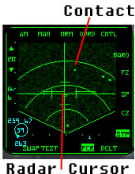
The radar displays the ground target modes differently to that of the air to air modes. Rather than distorting the radar returns into a b scope, the radar uses the arc style of scope instead, giving you a 'top down' view of the radar contacts. Once again range is represented by the relative distance up or down the scope in reference to the max range setting.
