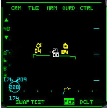
The track while scan mode is a unique and very useful mode that the AN/APG-68(V5) offers pilots. This mode enables pilots to get extra information from contacts that are within the radar cone. It can scan and track 16 targets at the same time, providing altitude, aspect, and heading and to some extent speed information.
