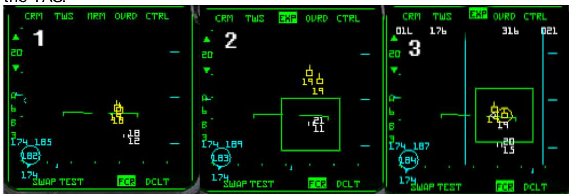
You can see whether the EXP mode is on by seeing if it is highlighted – if it is on it will flash. The EXP box will change in size depending on the radar range that is set, and is always to a scale 4nm.
