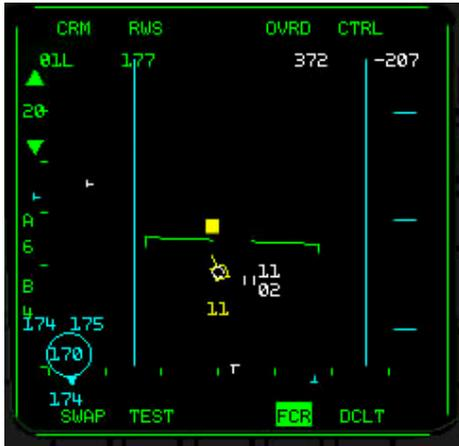
The situational awareness mode is a special sub mode that is designed to give more information on a specific target, but at the same time not remove the knowledge of the location of other contacts. Moving into RWR-SAM will increase the chances of the contact detecting you via a radar-warning receiver. However you do get a lot more information.
