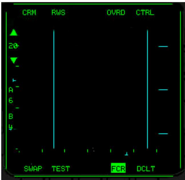
When operating in the restricted azimuth scan patterns, you can alter the horizontal direction that the radar is pointing by moving the Target Acquisition Cursors (explained later) left and right in the direction you wish the radar to look.
